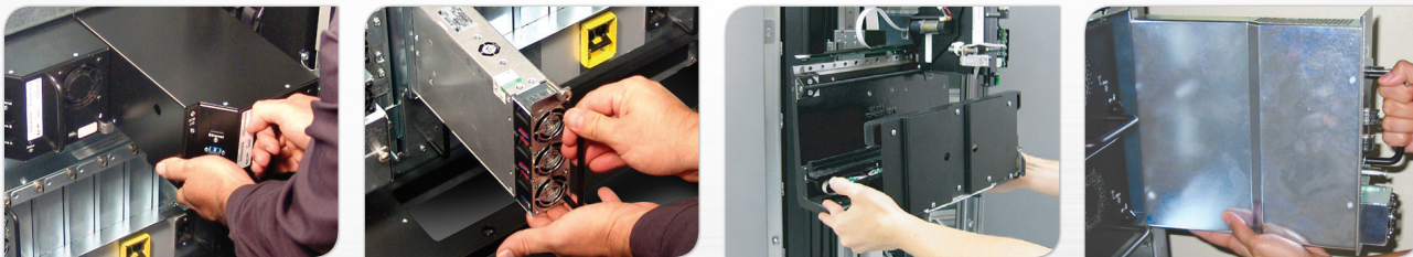
Drive → Power Supply → Robotics → I/O Blade (RIM)
